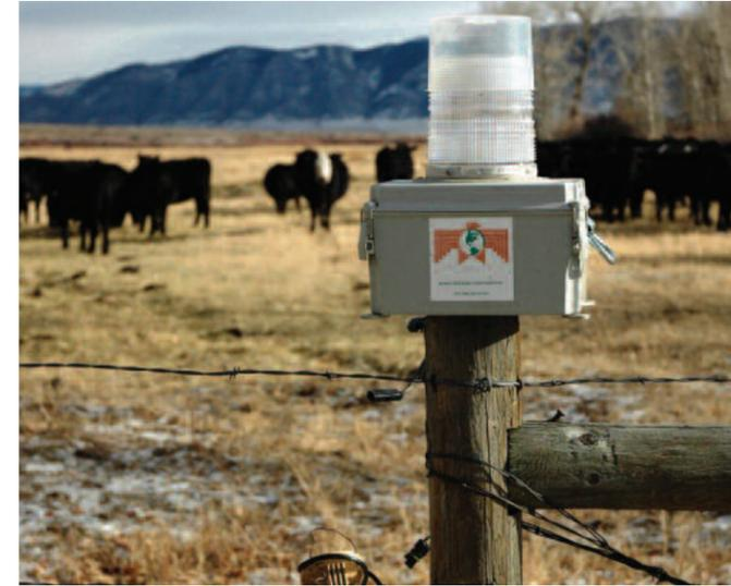
**Scare devices like motion or radio activated (MAG/RAG) boxes, sirens, strobe lights, pyrotechnics, scarecrows, and radios change wolf behavior by causing fear.**
